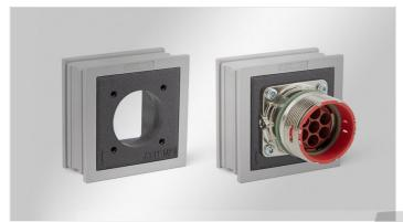
The grommet AT-FL is constructed on the basis of a large KT cable grommet. The polyamide body is moulded with elastomer. All square flanges with dimensions  $19.8 \times 19.8 \text{ mm}$  (M23) can be integrated.
