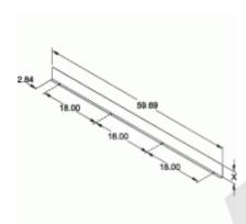
• Divides wireway into two or more compartments. Barriers are fastened to wireway sections with screws.
