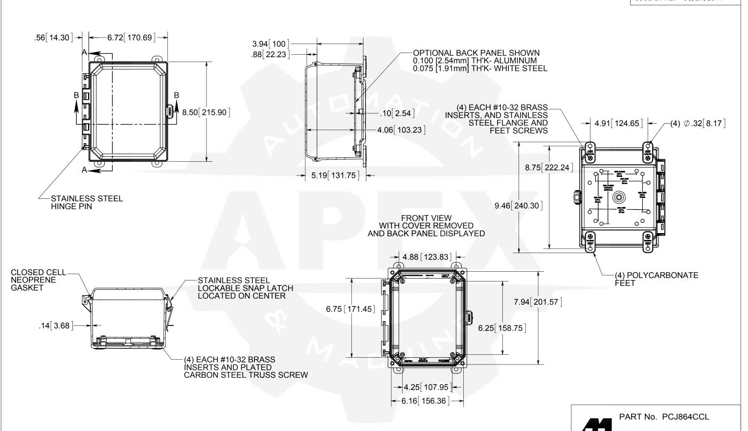
MATERIAL: BOX- INJECTED POLYCARBONATE STANDARD COVER- INJECTED POLYCARBONATE CLEAR COVER - INJECTED POLYCARBONATE
