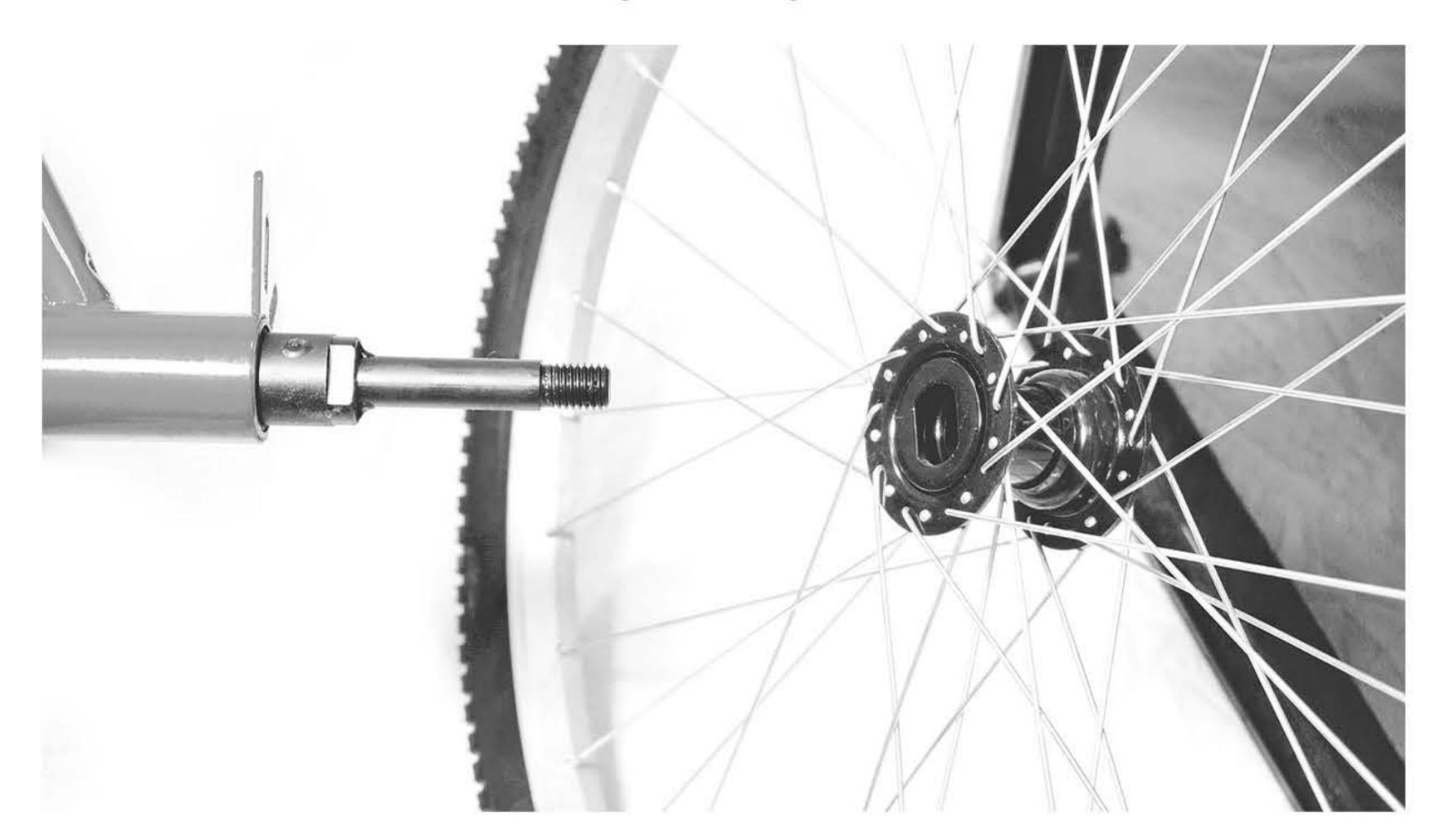
On the other side of the Rear Axle you will see a nut and a washer. Go ahead and remove both of these and slide on the other Rear Tire. Then put the washer and nut back on and fully tighten up the nut.
