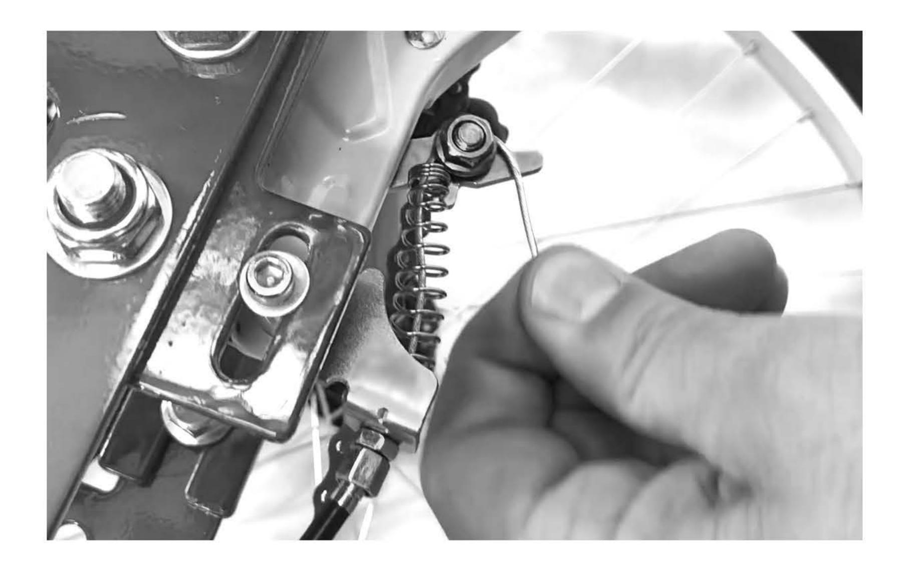
Then wrap the cable around under the nut shown here in the image. Finally tighten up the nut so the cable stays in place. You will need to put the bike upright again for the next step.
