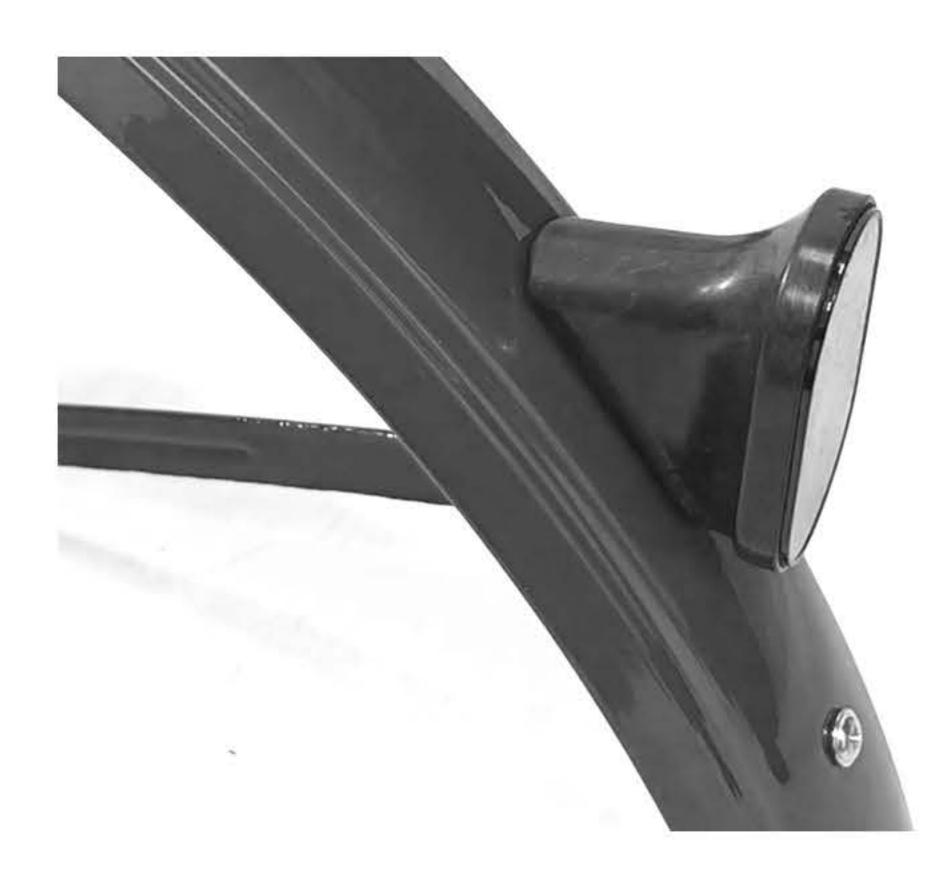
For the front reflector, unscrew the nut on the back. Then place the screw through the top hole and reattach the nut and tighten it.
