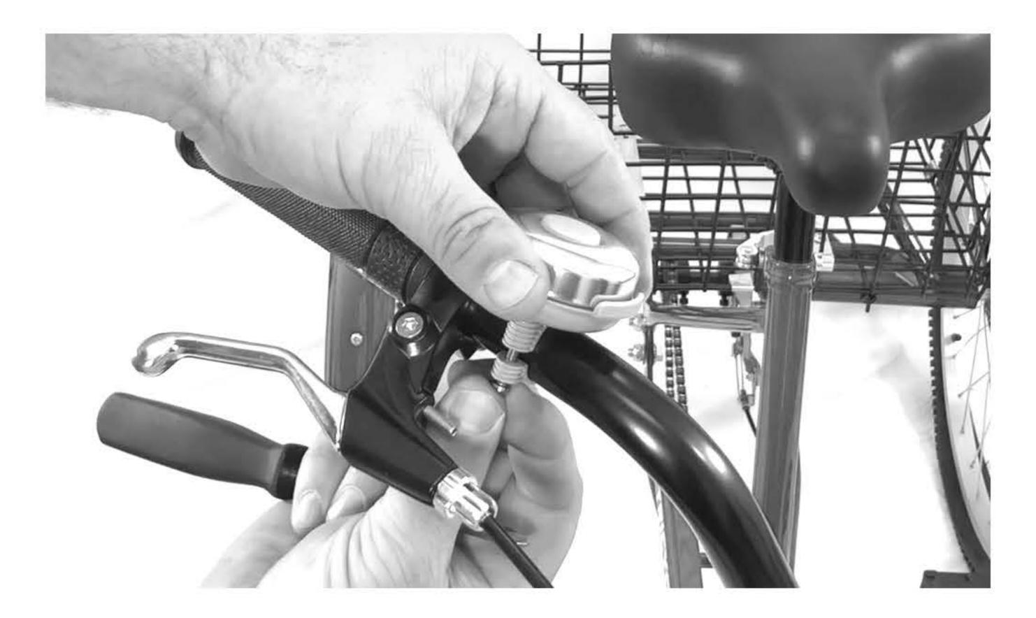
The final step you will want to take the small metal caps found in the bag. Placing one over the exposed wire of the front and rear brakes. Then with a pair of pliers, crimp the cap onto the wire.
