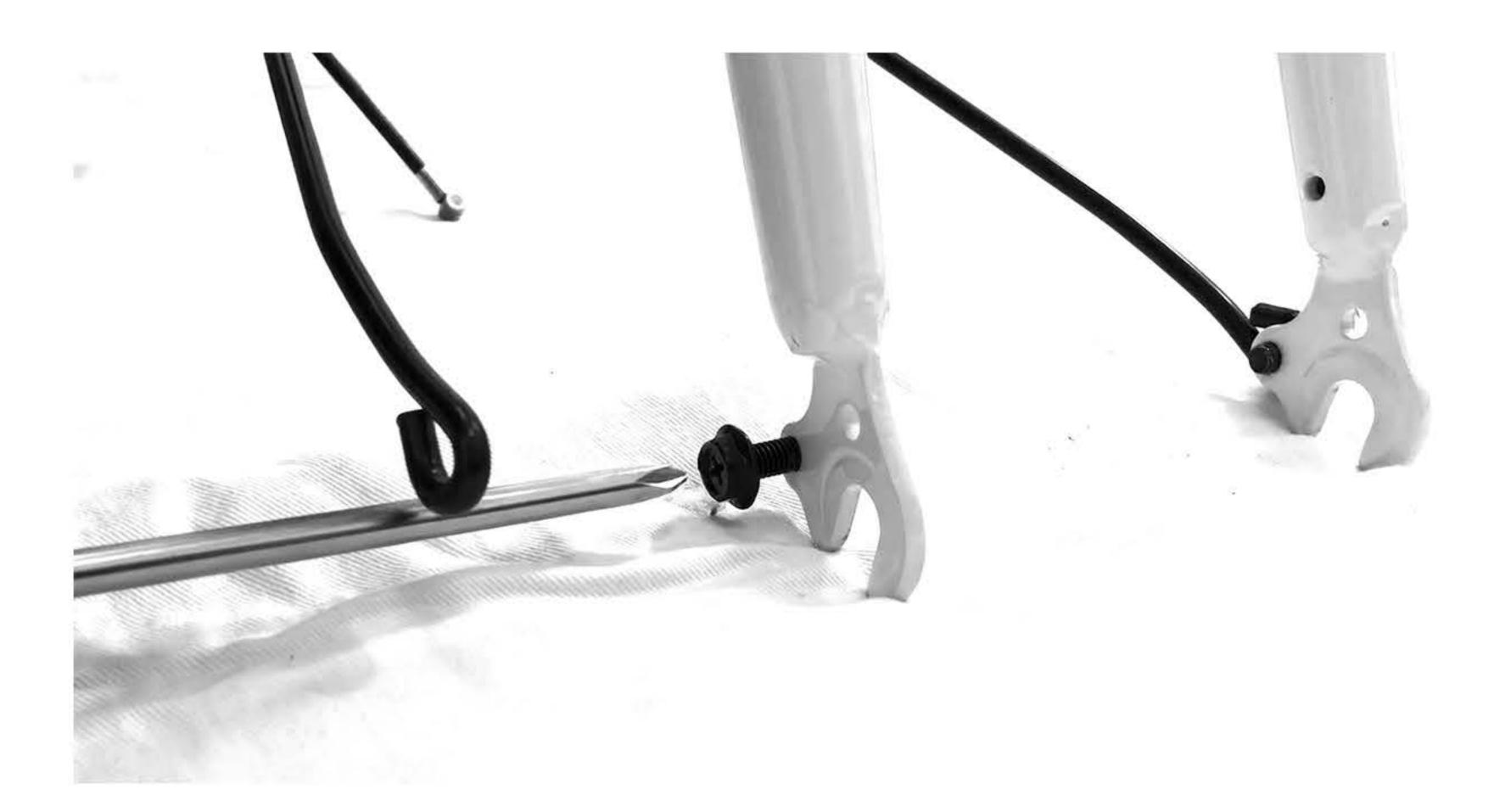
Now let's attach the wheel to the front. Start by sliding the tire in place on the front of the frame. Make sure that the washers with a latch on them are on the outside of the frame.
