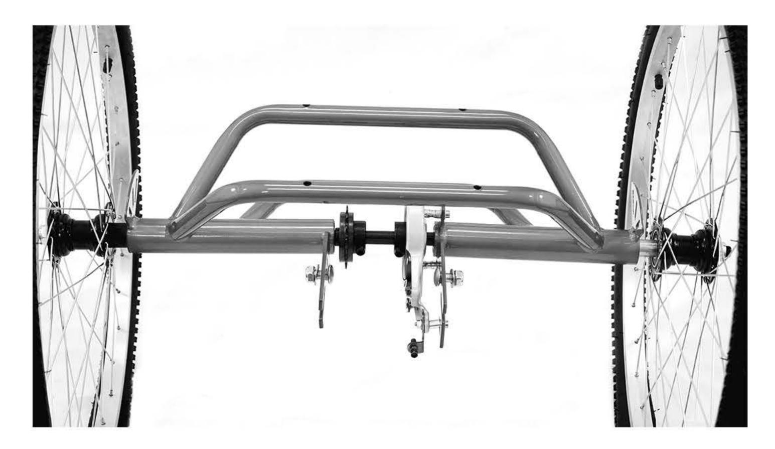
Next, we will be attaching the Frame to the Rear Axle. With the Frame in hand, slide it onto the Rear Axle with the bolts lining up into the grooves of both the frame and rear Axle. Do not tighten up the bolts just yet, this will occur in a later step.
