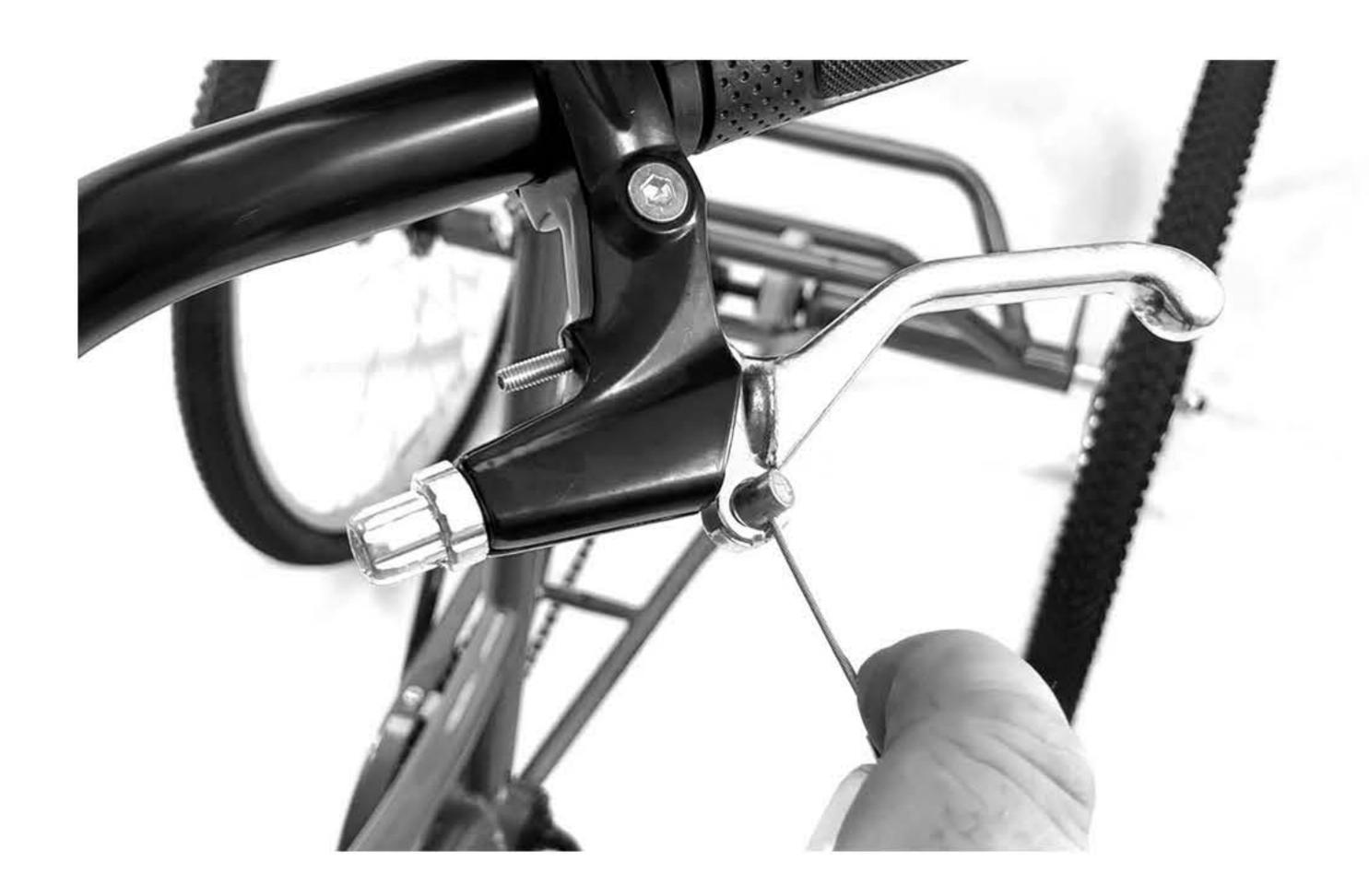
Then pull the lever and align the cable through the notch in the lever body. Repeat this for the other handbrake.
