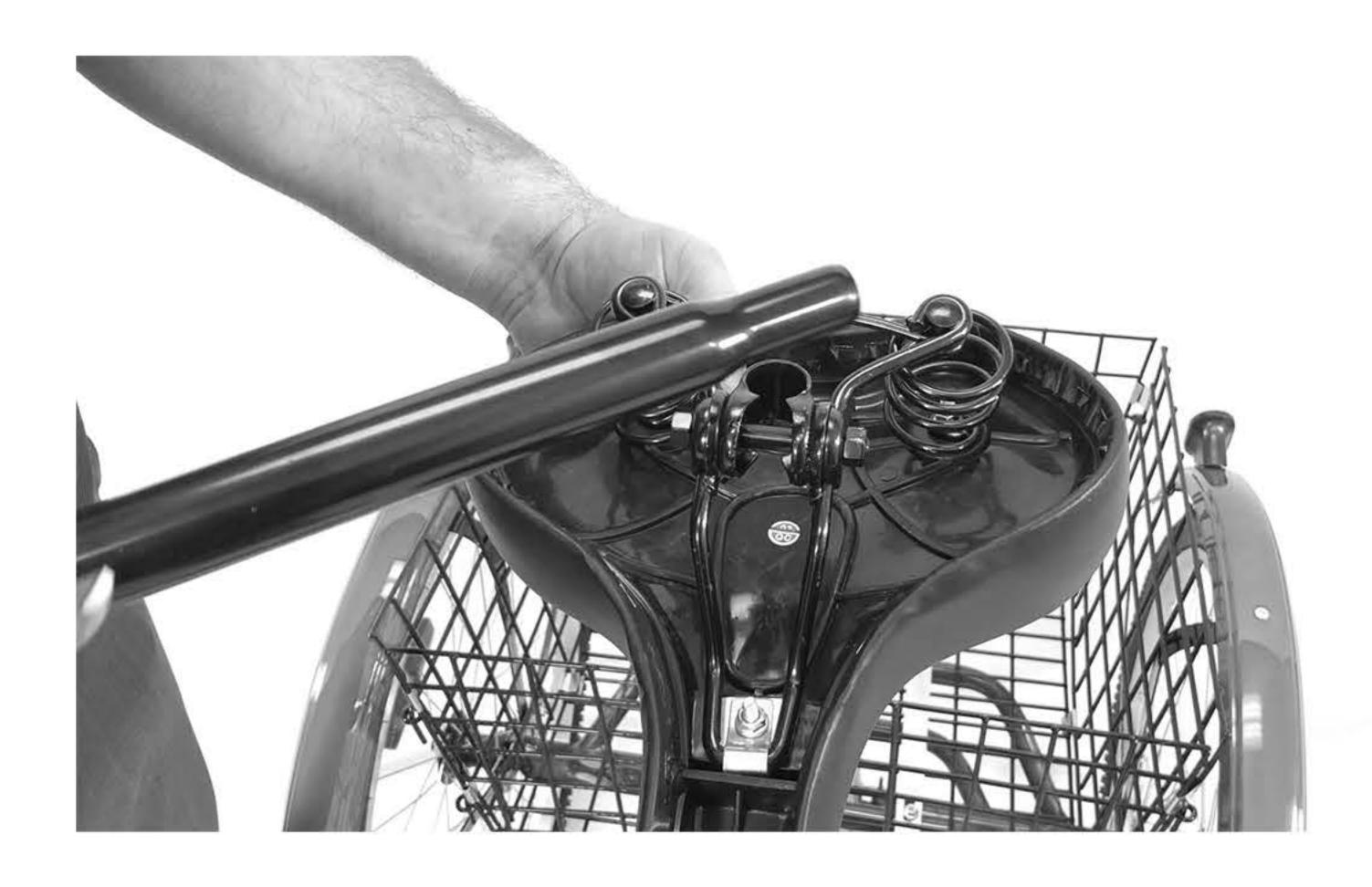
Then tighten the nut to secure the seat post in place. Now remove the protective cap on the frame. Rotate the latch to tighten up the frame for the seat post. Then insert the seat post into the frame and turn the latch to lock the seat in place.
