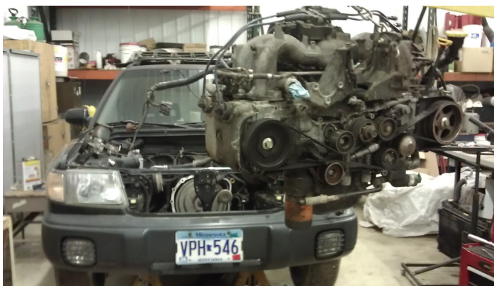
Seized idler on an interference engine; change your timing belt when it's due.
