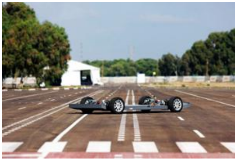
REE prototype platform for first phase of REEcorner TM and control technology validation tests for Navya's next-generation autonomous vehicles.
