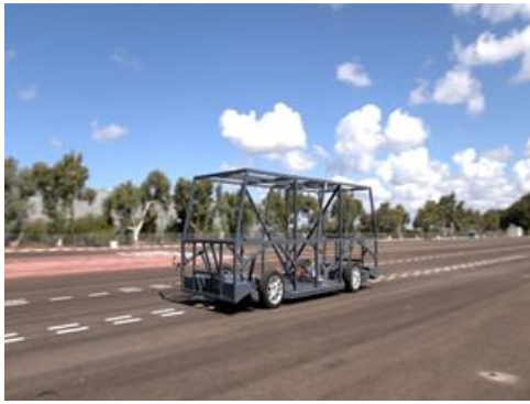
REE platform and frame that will be used to secure hardware such as lidars and sensors during completion of first phase of validation tests of REEcorner TM and control technology for Navya's next-generation autonomous vehicles.
