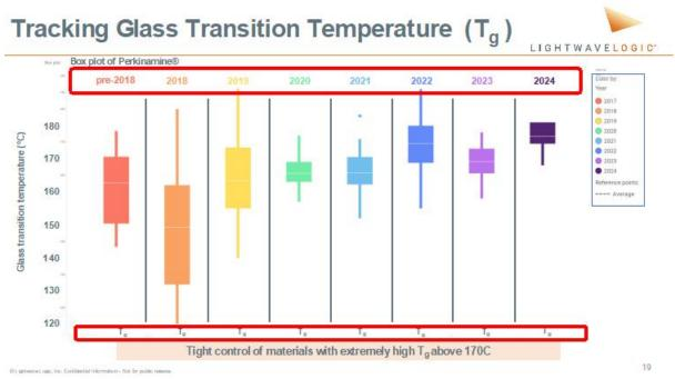
The above graphic shows the increasing trend of improved electro-optic chromophores that have been developed by the Company in respect to glass transition temperature. The graphic details improvements in Tg showing through the box plot extremely tight and improved material with Tg's above 170C with tight control of the materials performance as measured in thin films.
