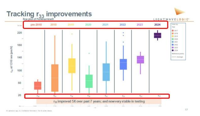
The above graphic shows the increasing trend of improved electro-optic chromophores that have been developed by the Company. The graphic details improvements in r33, a measure of electro-optic efficiency of Perkinamine® electro-optic material. The r33 has improved using a box plot, approximately over 5X during the past 7 years, and is now very stable in testing.
