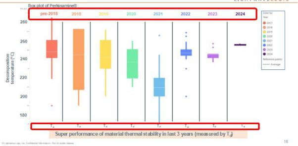
The above graphic shows the increasing trend of improved electro-optic chromophores that have been developed by the Company in respect to decomposition temperature. The graphic details improvements in Td showing through the box plot extremely tight and improved material thermal stability over the past 3 years, and excellent results over the past year.
