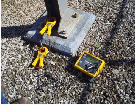
resistivity along with the ground grid system will identify abnormal conditions.
