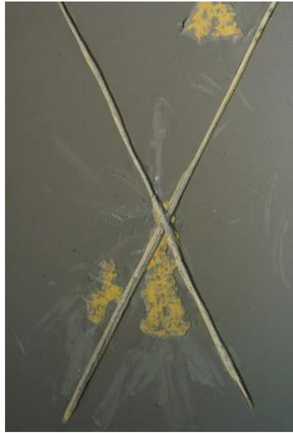
Paint Applied Over Grit Blasted Aluminum with Nanocomposite Pretreatment
