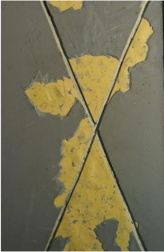
Paint Applied Over Grit Blasted Aluminum
