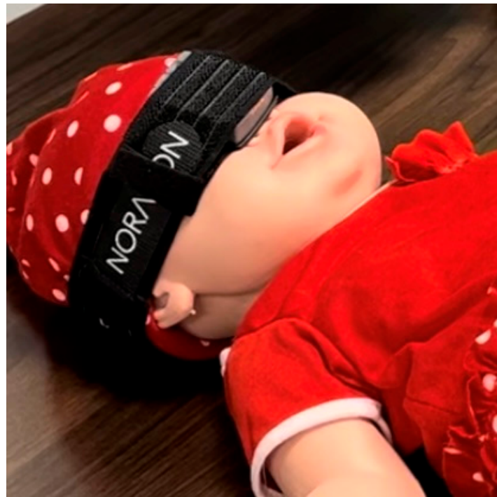
Figure 1. A photograph of the study design with an inertial measurement unit Velcroed around the silicone baby infant's head to determine the head acceleration during a non-recommended handling and head impact with a table.
