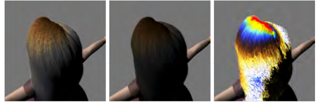
Figure 4: Unexpected behavior of a physically based shading model after some non-physical modifications to the underlying hair scattering functions. Left : A physically based setting for the shader will result in a reasonable multiple scattering component. Center : When the modified single scattering functions absorb energy the multiple scattering component might disappear. Right : When the single scattering functions produce energy, the multiple scattering component might blow up.
