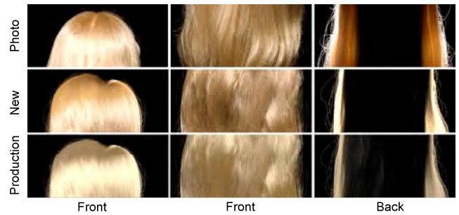
Figure 18: Comparing one of the results of the New shader (middle row) with one of the results of the Production shader (bottom row). Unlike the New shader, the Production shader fails to correctly produce the secondary highlight (left column), to capture the details of the light scattering inside the hair volume (middle column), and to produce the bright halo around the hair in the backlit situation (right column).
