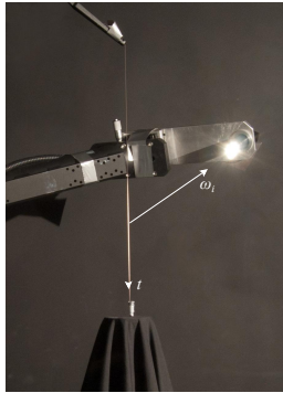
Fig. 7: The gantry setup used to measure the BSDF of threads. The thread is suspended vertically, which makes it possible to capture the full 4D BSDF.
