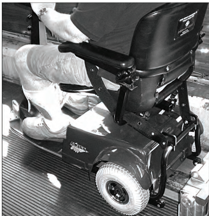
Figure 3. Amigo RD three-wheel electric scooter (Amigo Mobility International; Bridgeport, Michigan) equipped with two tie-down securement points, universal design interface geometry adaptor (UDIG), and UDIG-mounted pelvic restraint.
