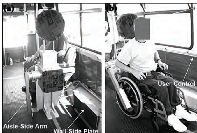
Figure 6. (a) Rear-facing wheelchair passenger station (RF-WPS) system with aisle-side arm and wall-side plate and (b) example of manual wheelchair positioned in RF-WPS.
