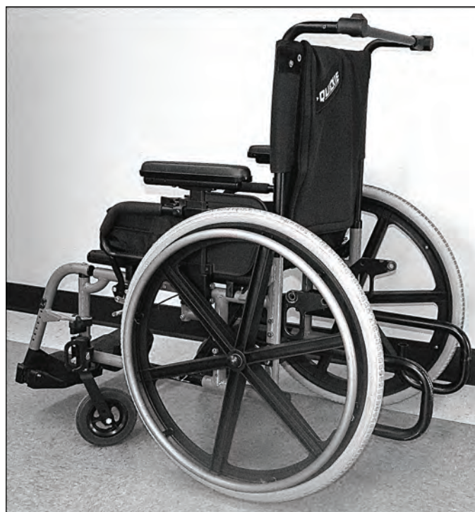
Figure 2. Quickie 2 manual wheelchair (Sunrise Medical; Longmont, Colorado) equipped with four tie-down securement points, universal design interface geometry adaptor, and frame-mounted pelvic restraint.
