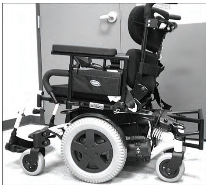
Figure 1. TDX SP power wheelchair (Invacare; Elyria, Ohio) equipped with four tie-down securement points, universal design interface geometry adaptor, and frame-mounted pelvic restraint.
