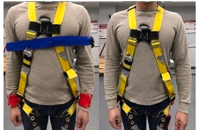
Fig. 2. Arm constraint positioning used in the current study with both arms constrained (left) and no arms constrained (right).
