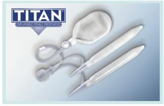
Figure 1. Photograph of Coloplast Titan™ inflatable penile prosthesis. Consists of paired inflatable Bioflex® cylinders, a scrotal pump and a fluid reservoir with autoinflation-preventing lock-out valve.
