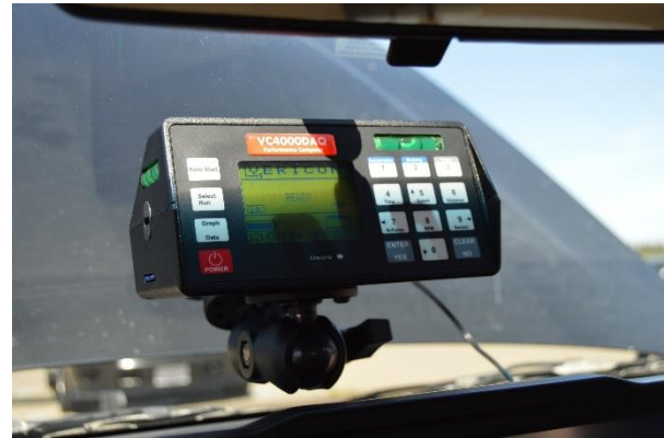
Fig 3. Vericom 4000DQA device mounted on the windshield.
