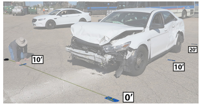
Figure 2. Placement of reference markers at specific distances alongside the vehicles.
