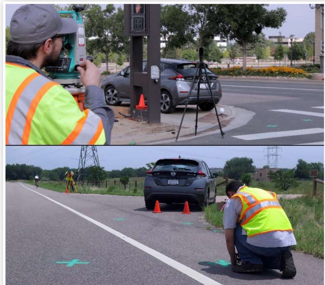
FIGURE 3 Recording locations of spray chalk and vehicle using a total station and 3D laser scanning.
