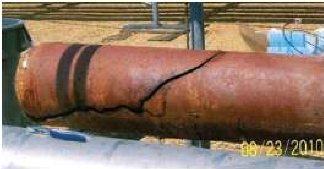
Figure 4. Pipe main ruptured by hydraulic shock (CSB Safety Bulletin photo from Millard incident).
