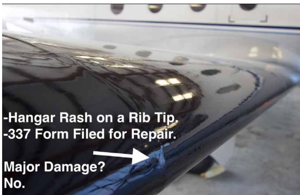
Photo 4. A "Major Repair" and the filing of a 337 Form does not always result in a Major Damage diminution in value. Appraisers must use their experience, knowledge, and discretion in these cases.
