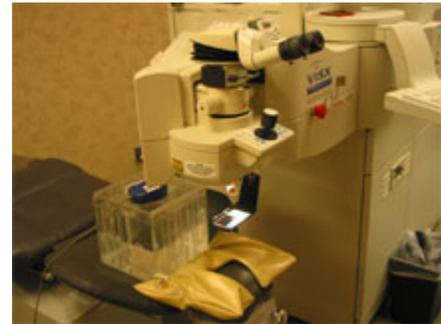
**Simulated thoracic chamber placed in patient position with a VISX Star S4 ophthalmic laser**
