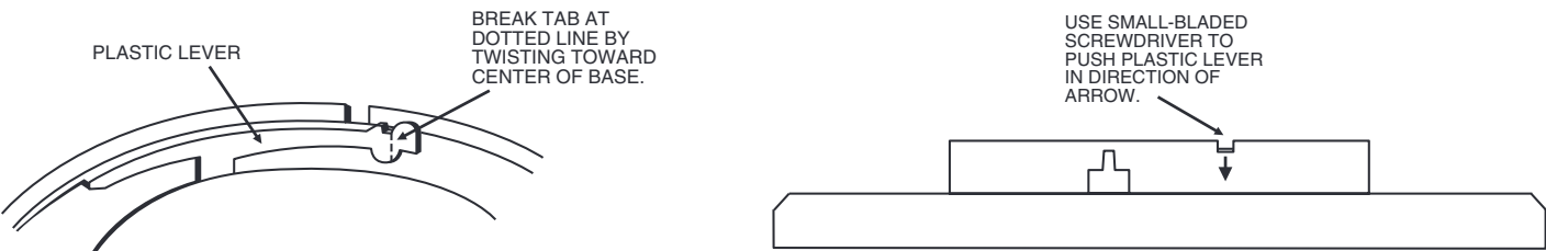
FIGURE 7B. REMOVING THE DETECTOR HEAD FROM THE BASE
