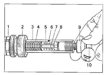
To fit the gauge to the advance device, remove the small plug from the spring cap (1) and fit the gauge body in its place. There is a small plug (10) from which any air may be bled before commencing testing.
