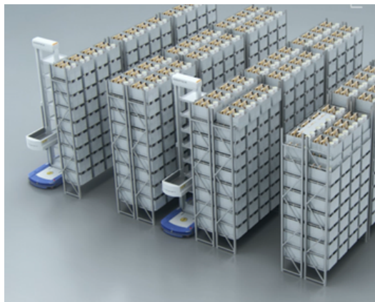
Robotics case-picking operations with thin 4ft wide aisles
