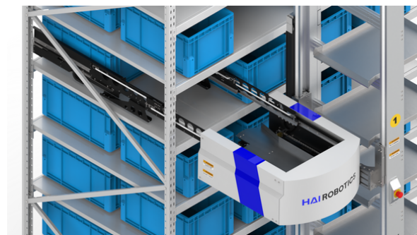
Robotics case-picking operations with thin 4ft wide aisles
