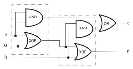
Wait! The figure has a misprint — an **or** where there should be an **xor**. In fact, either one works. Why is that? Here's the table for computing c' + c'':
