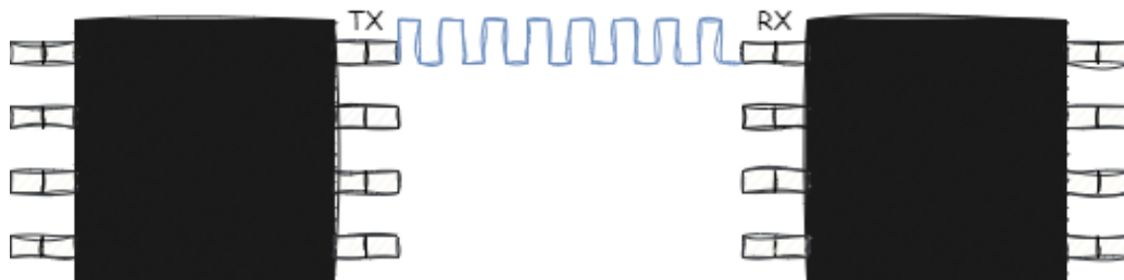
Figure 1.8 - Async communication protocol
