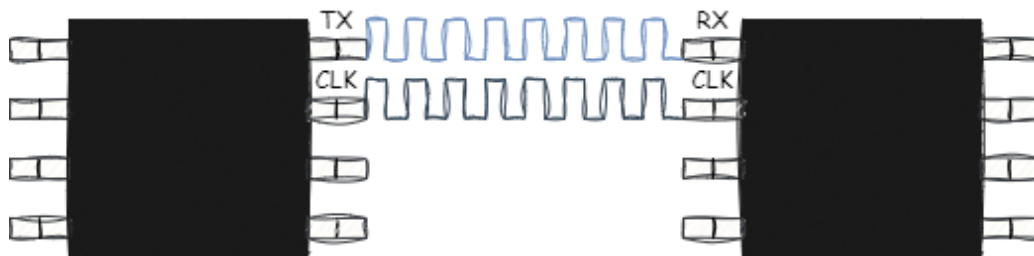
Figure 1.6 - Sync communication protocol
