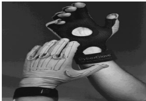
Figure C29: Glove that senses joint angles
