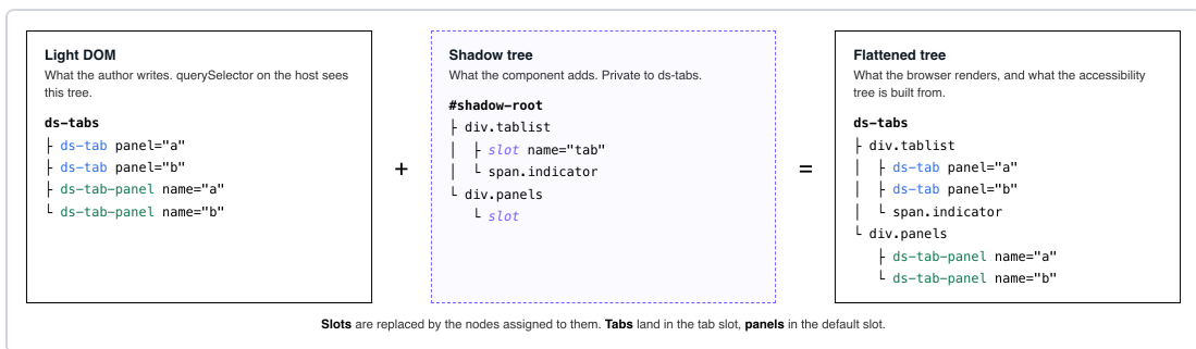
Figure 1-2. The light DOM and the shadow tree combine into the flattened tree
