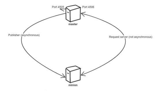
Let's now make sure that both components of Salt are able to communicate. Since the minion is the connection establisher, we need to check if the remote ports of the master can be reached from the minion.
