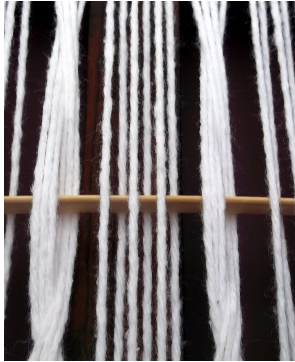
Showing the twist. This pattern is a combination of plain weave and leno.
