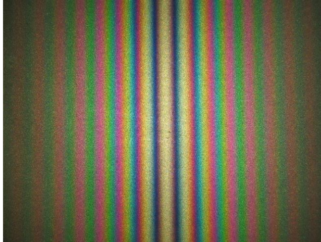
Figure 6. Interference pattern produced with a Michelson interferometer from Wikipedia https://en.wikipedia.org/wiki/Michelson%E2%80%93Morley_experiment
