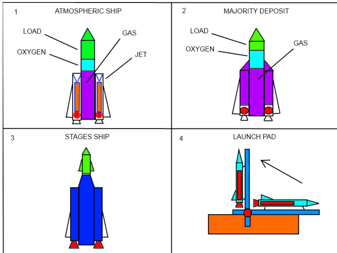
In the example number one atmospheric model ship is shown, this type of ship is single stage and has the advantage of carrying two turbojet engines that use atmospheric oxygen to accomplish the mission. This allows great fuel savings by not having to transport most of the oxygen.
