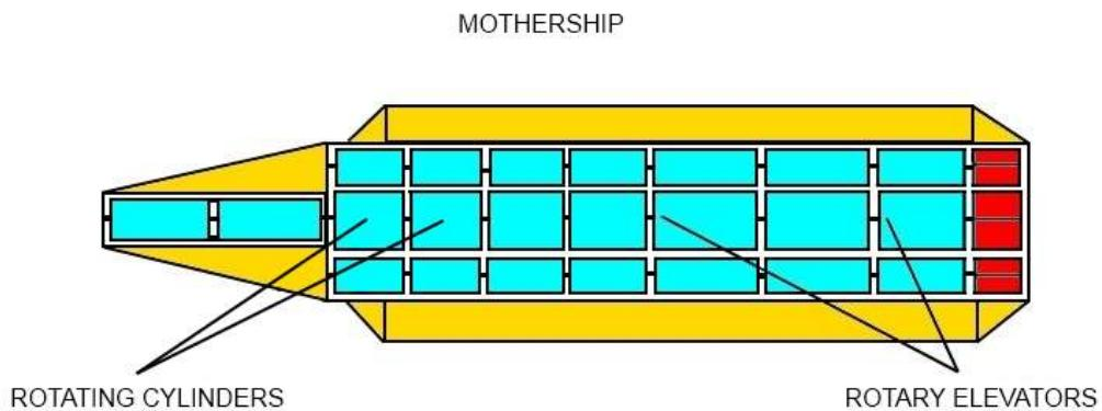
In this scheme we can see how it would be a mother ship view from above, it can be seen that the rotating cylinders are placed inside the helmet and parallel to the path of the ship, thus position is prevented by a side movement cylinder impact on the stability of the outer shell, and on the other prevents spurts or braking destabilize the inner gravity.
