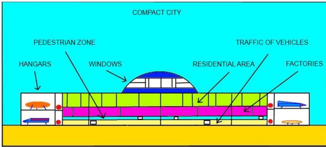
In this type of city transport vehicles would use the lower section. Located above section would be used for pedestrian traffic, to avoid the risk of abuse. On top of this section would be the area of factory and office work. Finally above all would be located residential areas where housing would be found.
