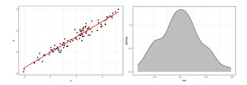
The left graph shows how the residual variable is calculated, while the one on the right shows its observed distribution (or density).
