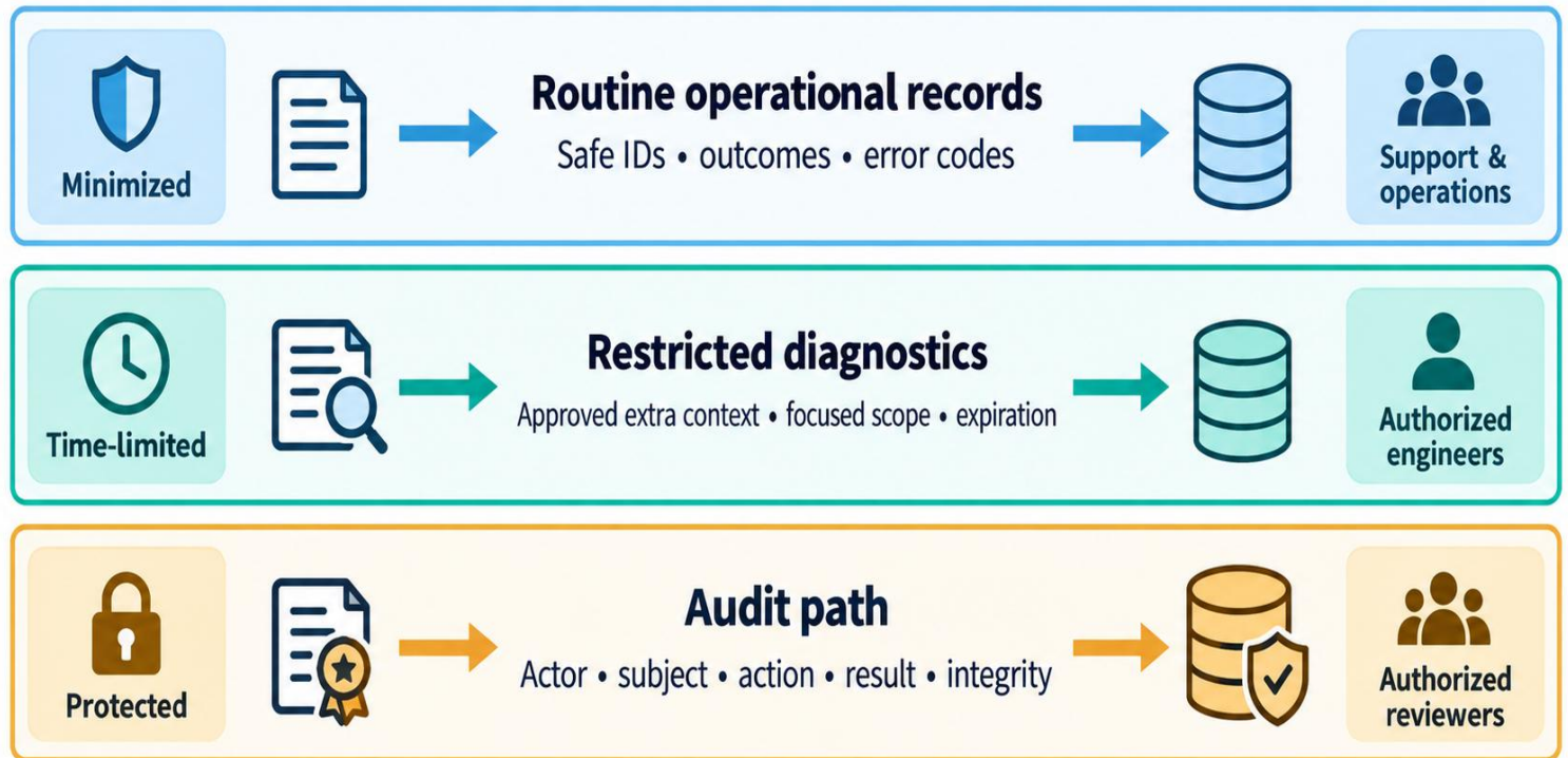
Figure 2-7: Resolving conflicting requirements with layered evidence
