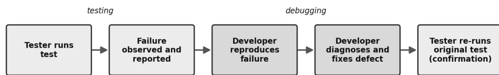
Figure 1: Flow from a tester running a test and reporting a failure, through a developer reproducing, diagnosing, and fixing the defect, to the tester re-running the original test for confirmation.
