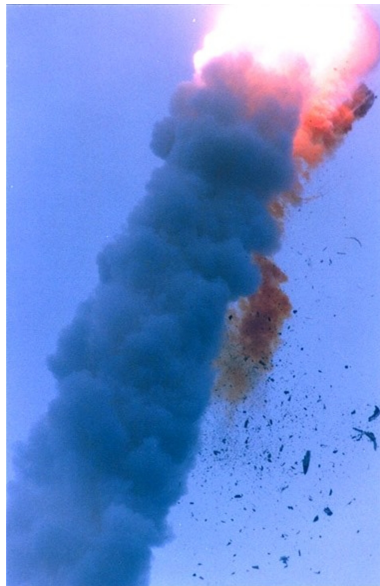
Figure 2: Ariane explosion was caused by buffer overflow
