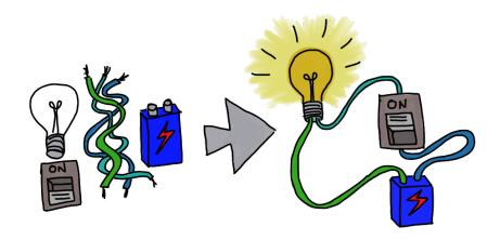
If we connect these components into a circuit by binding them together, we can throw the switch (that is, give the circuit some input) and the light bulb
