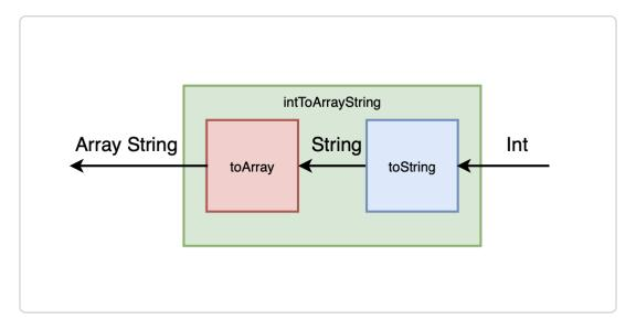
toString takes an Int and outputs a String, which is the input to toArray that outputs Array String.
