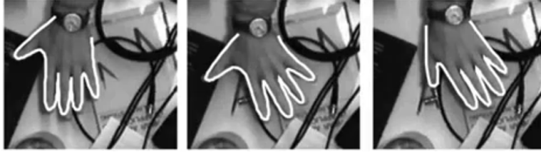
Figure 12.7: Tracking the movement of a hand using an edge detector.
