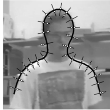
Figure 12.8: A contour and its normals. High-contrast features (i.e. edges) are sought out along these normals.
