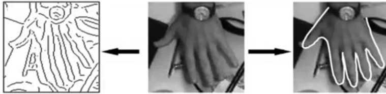
Figure 12.9: Using edge detection and contours to track hand movement.
