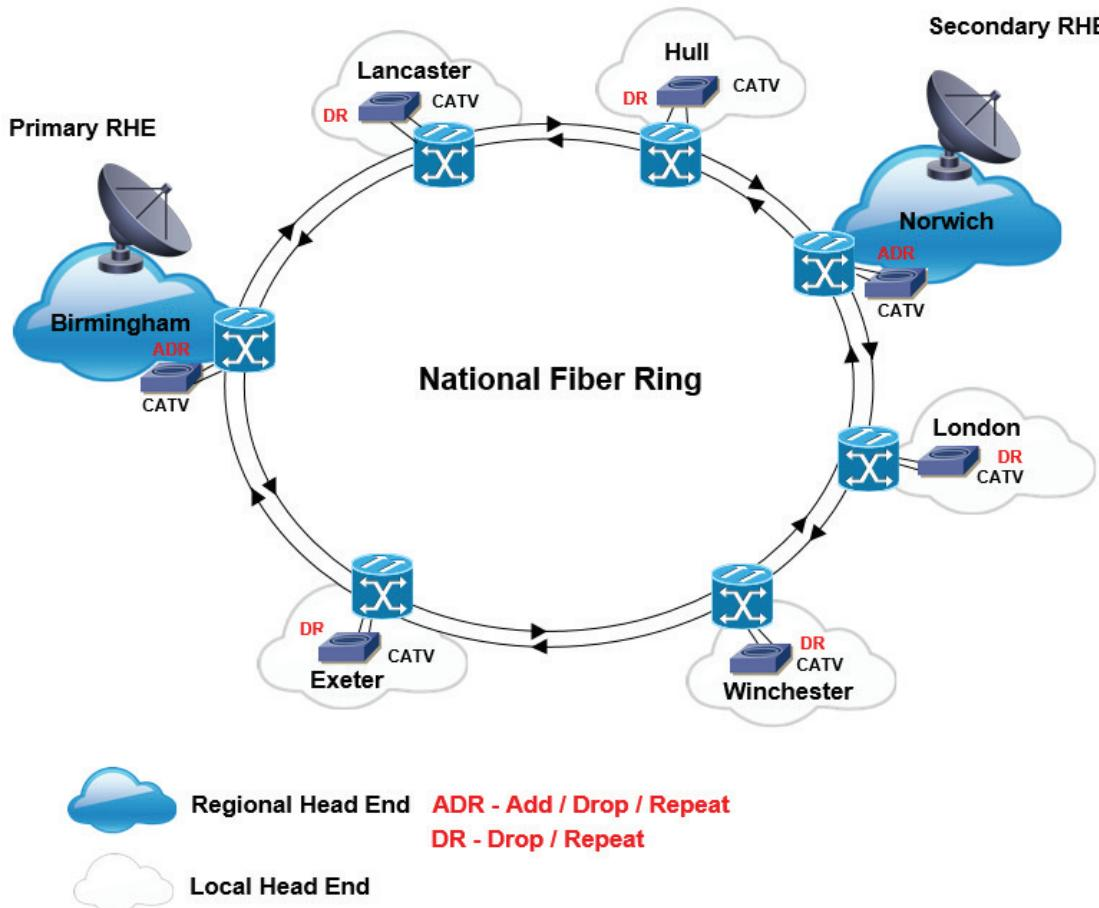
The following figure details the “Add” functionality of a primary RHE and the “Repeat” functionality of an LHE for Channels onto the Ring, although “Drop” capability is provided within LHEs this functionality is not currently utilised. The primary RHE is shown to drop the signals on Channel Input as these were the original signals transmitted to the ring which have returned and would otherwise cause a looping of traffic around the ring.
