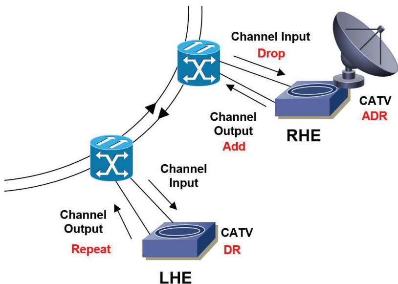
When new LHEs are added to the network the existing fiber ring is expanded from the closest existing LHEs to the new LHE location and then the ring is re-joined with the then redundant fiber circuits decommissioned. This procedure is not disruptive to the network due to the SONET protection in place but it has proved to be financially challenging due to cost of dark fiber runs. The procedure is outlined in the following diagram for when the Lancaster LHE was added to the network:
