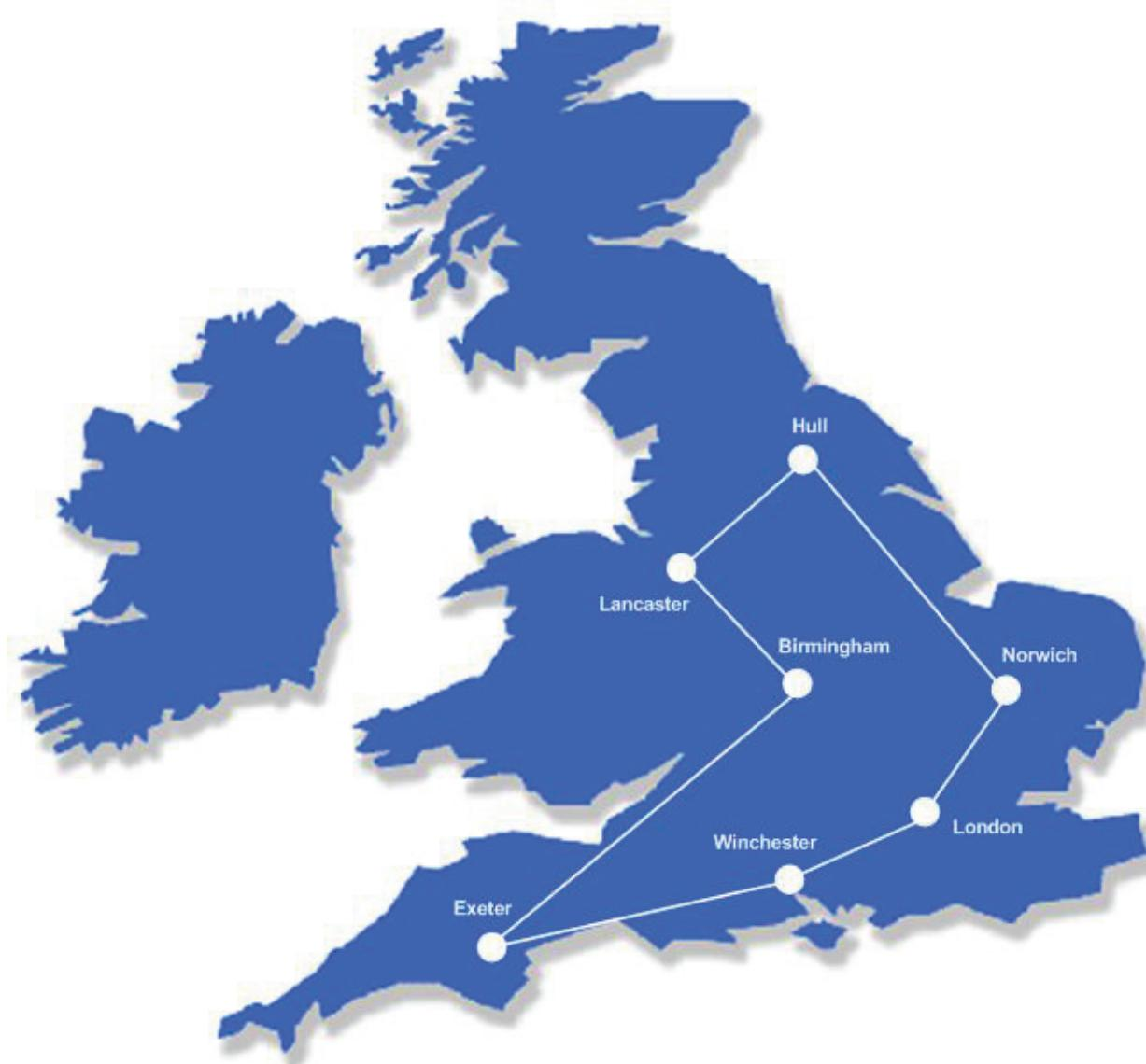
Diamond TV was formed in 1993 and provide Cable TV, Internet & Telephony services to residential customers from their national dual fiber ring running around the North and South of the UK. The ring is constructed of a clockwise and counter clockwise ring from dark fiber, it is owned outright by the company and operates as a protected SONET OC-192 dual ring.
