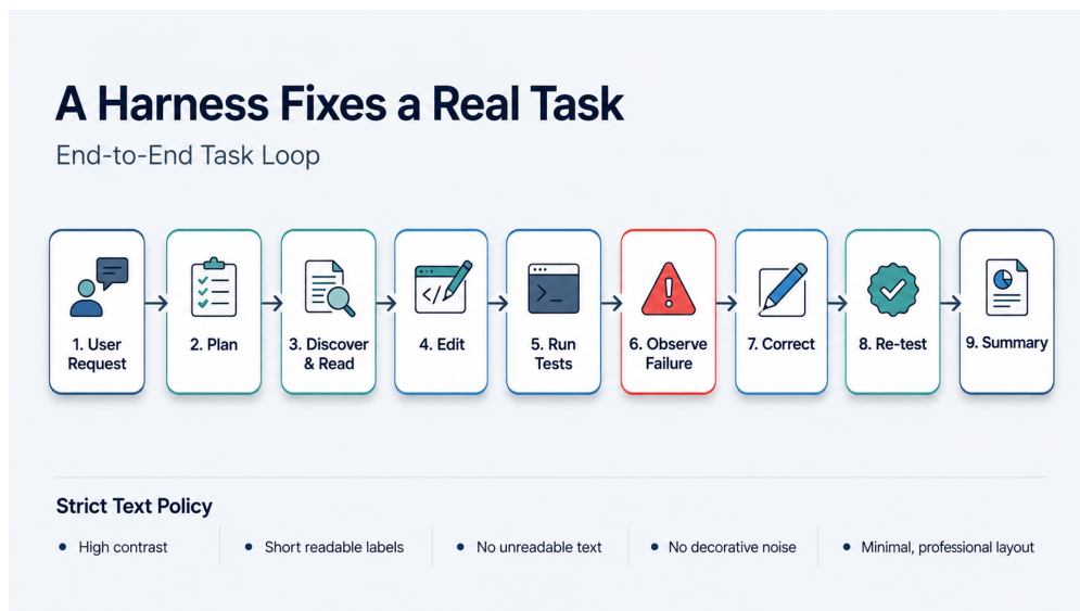
Figure 1.3: A harness does not merely answer once; it loops through planning, tool use, observation, correction, and verification until the task is complete.
