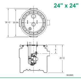
\* For 2" sewage ejector retrofit, simply remove and discard basin. Cover and suspended grinder pump will drop into existing basin. Cover may require field alignment to support reduced debris build up.
