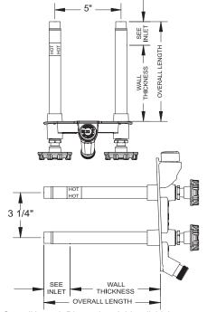
Overall Length Dimension: Add wall thickness and inlet option length shown in chart on reverse side.
