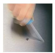
It happens time and time again that the tip slips out of the screw screwdriving, head when sometimes damaging valuable surfaces or even causing injury. The tips of the Wera Lasertip screwdrivers are microscopically roughened by means of a laser. This rough surface literally "bites" itself firmly into the screw head. Slipping out becomes a thing of the past.
