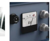
Our screwdrivers are tested for dielectric strength under a 10,000 volt load to make sure that their most important property, their insulation, has been exhaustively tested. Each individual Wera VDE screwdriver is subjected to this
