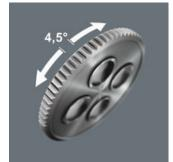
The Zyklop VDE ratchet allows a short return angle of only 4.5  $^{\circ}$  thanks to its 80 teeth.
