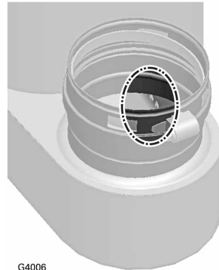
Figure 84 Recuperator flueway drain holes
