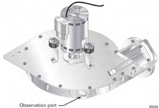
Figure 72 Check for igniter glow by looking into observation port on front of blower housing
