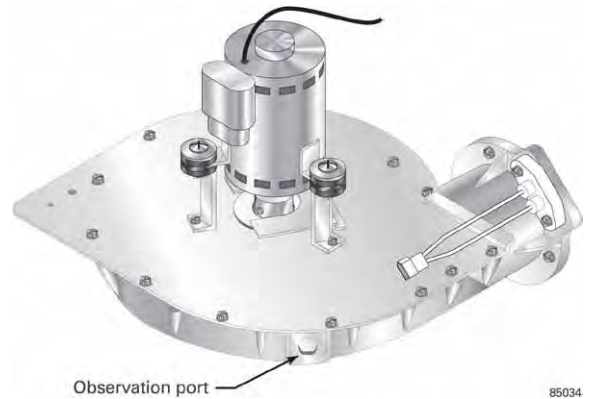
Figure 78 Igniter observation port in blower
