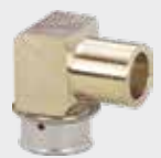
Viega PureFlow Press 90° elbow Zero Lead - Bronze - Press connection, street, female copper tube size Note Copper connection can be used as either male or female connection. Model 2814.7ZL
