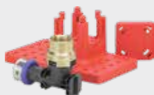
Viega PureFlow Press 90° elbow Smart Connect technology, Zero Lead - For fire sprinkler systems - Polymer - Press connection, female pipe thread Components Mounting bracket Note For use with black Viega PureFlow PEX only. UL listed for NFPA 13D systems Model V5645ZL
