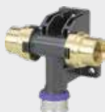
Viega PureFlow Press wall tee Smart Connect technology, Zero Lead - For fire sprinkler systems - Polymer - Female pipe thread, press connection Note For use with black Viega PureFlow PEX only. UL listed for NFPA 13D systems Model V5641ZL
