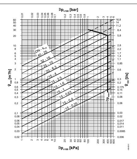
Maximum permissible differential pressure across the valve's control path, valid for the entire  $\Delta p_{max}$ actuating range of the motorised valve
