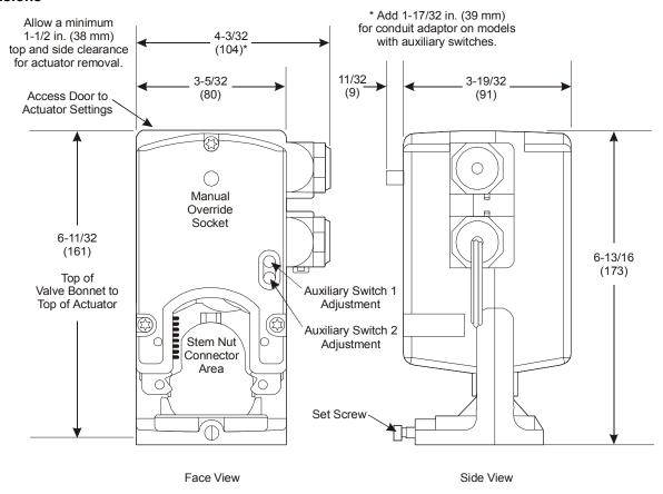
Figure 1: Actuator Dimensions, in. (mm)
