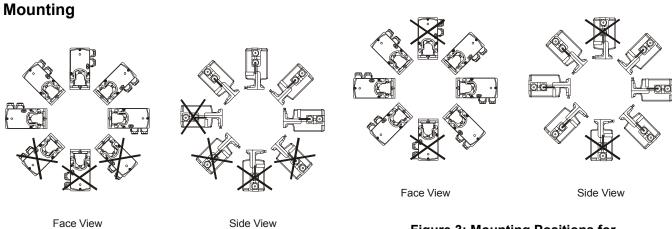
Figure 2: Mounting Positions for Chilled Water Applications and Condensing Atmospheres
